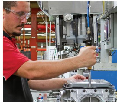
A six-speed front-wheel-drive transmission being assembled at DSIH's Albury plant in New South Wales.
